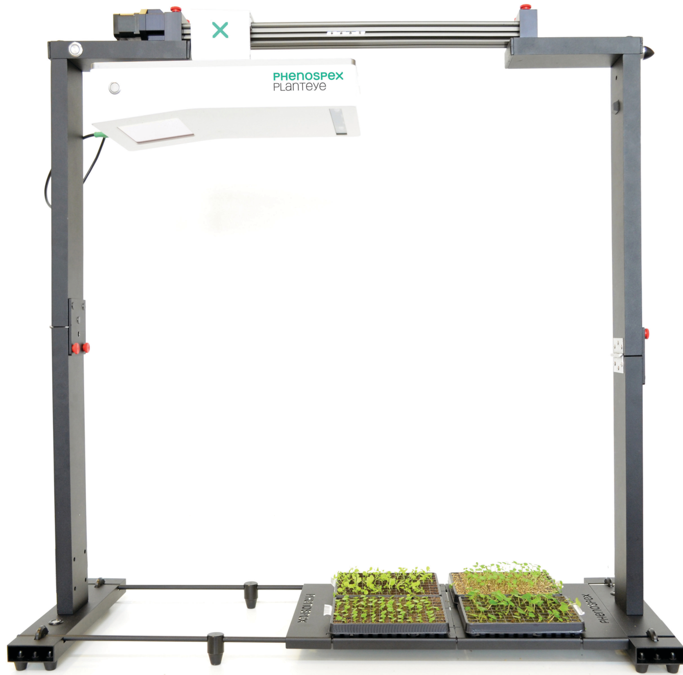
Fig. 1: Assembled MicroScan. The PlantEye F500 sensor allows for 3D and Multispectral imaging.
