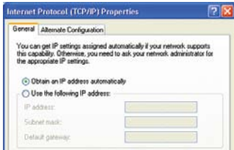
Figure 8-8: Internet Protocol (TCP/IP) DHCP Addressing
