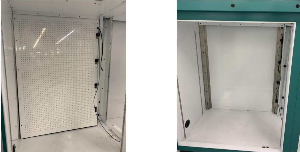
Figure 3-23 Remove The Plenum
