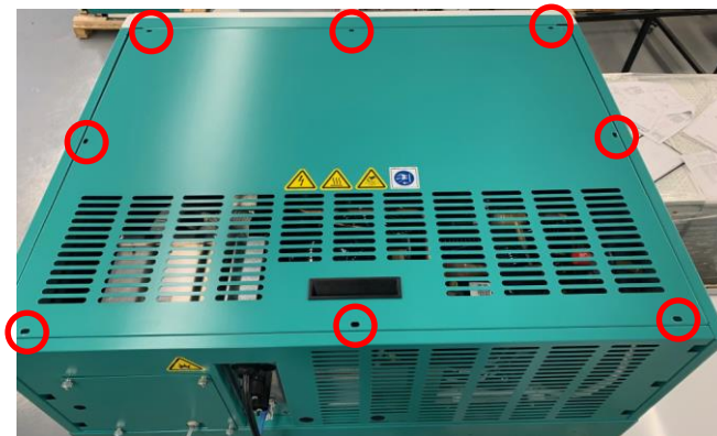
Figure 6-2 Remove the Screws from the Top Cover
