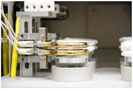
ColdBlock<sup>TM</sup> Digestion systems, discovered and manufactured by ColdBlock Technologies Inc., is a new sample digestion technology that dissolves solid matter into a solution for multi-element analysis. The technology is the first to use short-wave infrared radiation (IR) utilizing IR lamps and a cold block to perform sample digestion. The high energy radiation produced by the IR lamps is absorbed directly by the sample particles in an acid medium, generating much higher
